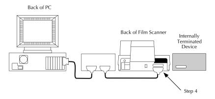
5. Attach the Scanner to the internally terminated device by plugging one end of your 50-pin to 50-pin SCSI cable into the empty SCSI port on the Scanner and the other end into the empty SCSI port on the terminated device. Seat both connectors firmly and pinch both wire clamps shut.
